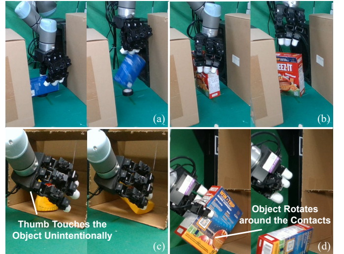
Fig. 8: Failure cases in real-world experiments. (a-b) The quality of a small subset of generated grasps is degraded by the guidance, leading to unstable grasps holding only the object's edge. (c) The dexterous hand unintentionally contacts the object due to open-loop execution. (d) The object shifts in hand because of inaccurate mass parameter estimation or insufficient friction.
